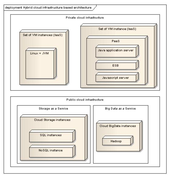
Figure 31 Hybrid Cloud infrastructure based architecture
